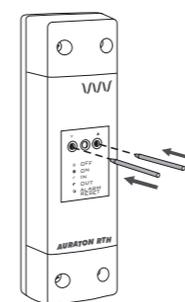
In order to sign out all devices associated with the receiver press and hold at the same time both association and sign out buttons ( ▼ and ▲ ) for at least 5 seconds until signalling of the LED diode changes to alternate flashing in the green and red colours. Then release both buttons.
