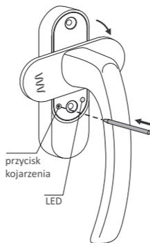
2. When the LED diode of the receiver flashes with a green light "the association button" should be pressed on the **H-1** handle (located under the cover) and held pressed for at least 2 seconds. When the LED diode on the handle starts flashing with a red light we release the button.
