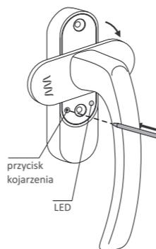
2. When the LED diode of the receiver flashes with a red light "the association button" should be pressed on the **H-1** handle (located under the cover) and held pressed for at least 2 seconds. When the LED diode on the handle starts flashing with a red light we release the button.
