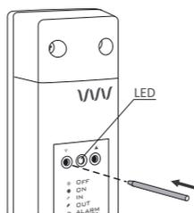
1. Associating the **H-1** handle with the receiver is initiated by pressing the left association button (green triangle - ▼) on the receiver and pressing it for at least 2 seconds. until the LED diode starts flashing with a green light, then we release the button..
