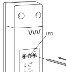
1. Signing out the **H-1** handle from the receiver is initiated by pressing the right signing out button (red triangle - ▲) on the receiver and pressing it for at least 2 seconds until the LED diode starts flashing with a red light, then we release the button.
